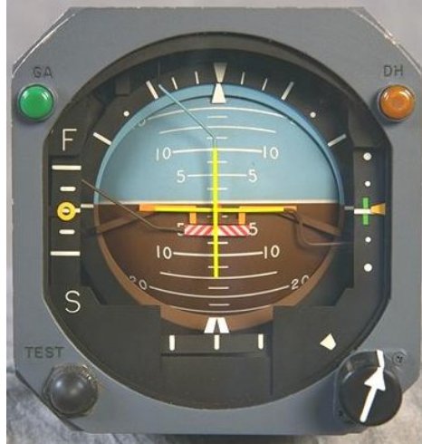
Figure 1. Airplane attitude indicator. The top portion of the background is blue and the bottom portion is brown. Lines in the middle of the display are fixed in the foreground and resemble the cross-section of an airplane. When the airplane cross-section is in the blue part of the background, the airplane is heading up into the sky. When it is in the brown part, the airplane is heading towards the ground. (Photo source: Wikimedia Commons: http://en.wikipedia.org/wiki/File:VMS_Artificial_Horizon.jpg )
